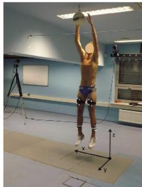
Fig. 1. Experimental setup, with a subject wearing passive reflective markers.
